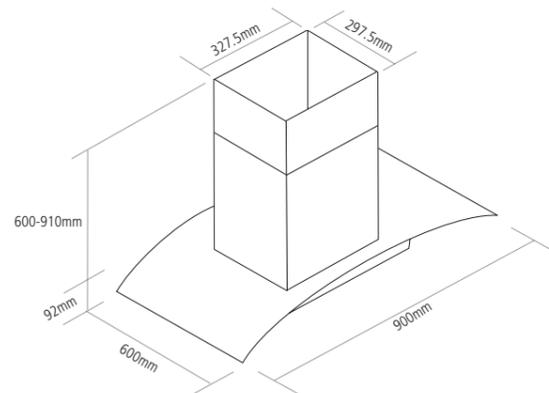
Note: Suitable to be installed in a standard room height of 2.3m
