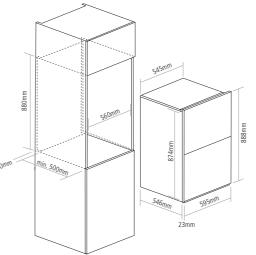
We recommend that when installing a stack or quad of products, a pair of our installation brackets [OVEN/BRACKETS2] are purchased to support the upper product ensuring a seamless fit for each appliance when one is on top of the other.
