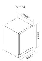
Ventilation requirements - Please allow an 127mm gap around the whole appliance when installed next to a wall, unit or in an alcove
