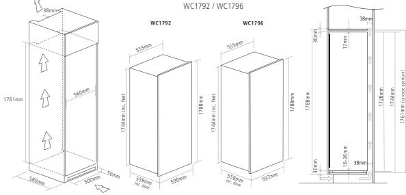
Please note: once installed the appliance door may not sit completely flush with the kitchen furniture door. Dimensions may vary +/- 2mm due to manufacturing tolerances
