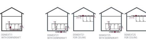
DUE TO THE POWER AND FITMENT OF OUR EXTERNAL MOTORS, RIGID DUCTING MUST BE USED.
