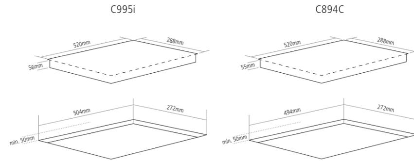
If installed without a gap in between, cut-out width = [no. of hobs - 1] x 288mm + 268mm
