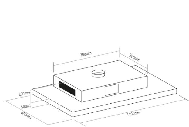
For installation create a false ceiling with a round niche of 510mm, with a minimum height of 220mm.
