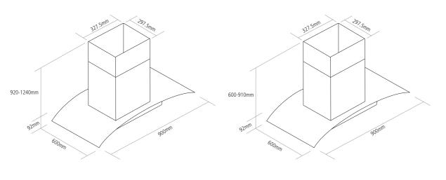
Note: Suitable to be installed in a standard room height of 2.3m
