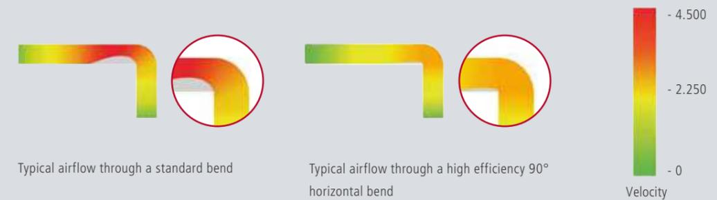
Typical airflow through a standard bend
